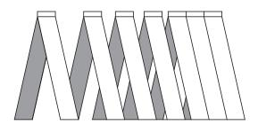
The AA STOOL is characterized by its simple design, using only 26x87 mm wooden profiles. Usually two "A trestles" form the AA STOOL (A+A = AA) – but they can also be used individually, in small rooms or when guests arrive. Stacking is also possible and stimulates the imagination for further uses.
